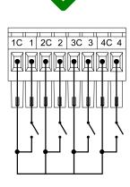
Wiring together common terminals within the same input block: **OK**
