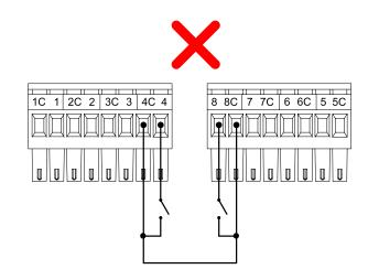
Wiring together common terminals from different input blocks: **NOT OK**
