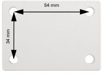
Fig. 10 Hole diameter 6.2 mm
