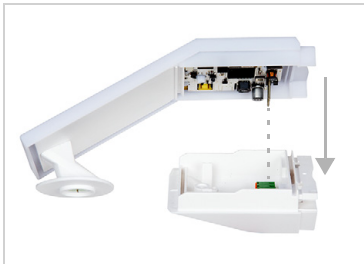
Fig. 15 Push the lid on the lower part. This also makes the plug-in connection between the board in the lid and the socket in the lower part.
