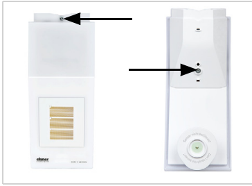
Fig. 6 Slacken both screws on the lid (top) and lower part (bottom) with a size 6 Torx screwdriver.
