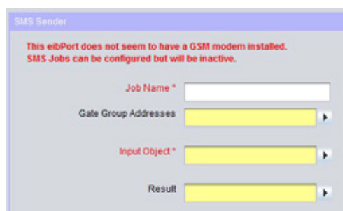
Figure 129: Job mask – GSM Modem not implemented / not detected
