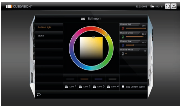
Extended Control Panel (ECP): Selection of lighting colours and scenarios
