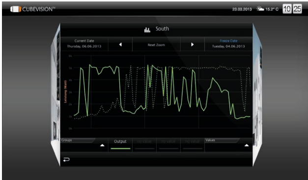
Extended Control Panel (ECP): Representation of the performance of a PV system
