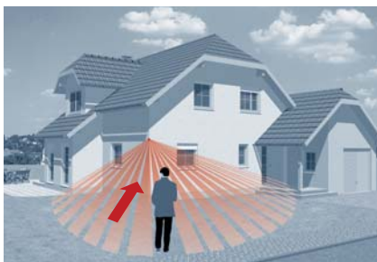
Radial detection – movement directly towards sensor (detection reach less than normal reach)
