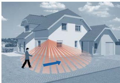
Tangential coverage – movement across the sensor detection zone (nominal reach)
