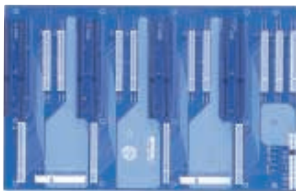
BPAS-PCIS-17 (4 segments \triangleq 4 IPC in only one chassis)
