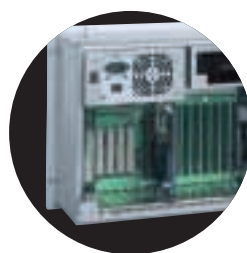
up to 13 free slots, easily accessible by dismantling card clamps
