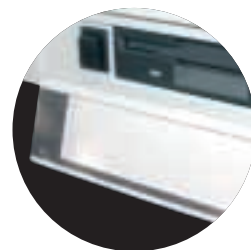
FDD, CD-ROM, PS/2 port, behind protection cover
